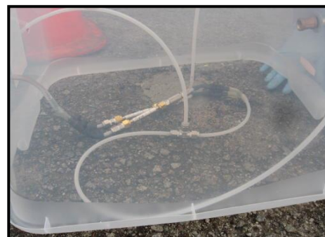
Sample collection with sorbent tube
