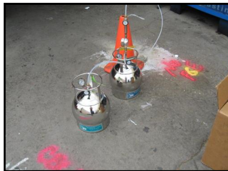
Sample collection with Summa canisters
