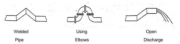
Full-pipe problems occur less frequently in pressurized systems. When they do, they are usually associated with the failure of an air relief valve. The best protection against this potential problem is, if possible, to locate the air relief valve downstream from the meter.
