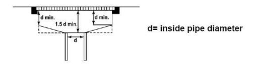
All covers must be installed according to the manufacturer's specifications. Provide a sump as specified by the manufacturer. Some covers do not require a sump, but may require they be installed with a special mud ring or other attachments. Please be aware that covers may need to be replaced after 3 to 10 years. Most covers have a life span of 5 years. Always replace broken or damaged covers.
